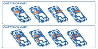
Place the SIM card with the chip facing downwards and slide it into its housing. Make sure that it is correctly inserted. To remove the card, press and slide it out.
