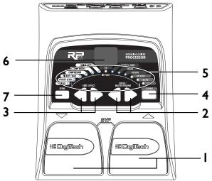
1. Footswitches - These 2 Footswitches are used to select presets, access the Tuner, or bypass the RP55. The Up Footswitch increments, and the Down Footswitch decrements through the presets. Pressing both Footswitches simultaneously bypasses the selected preset. Pressing and holding both Footswitches accesses the Tuner.
