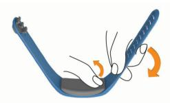
2 Insert the module into the replacement band. The device key on the module must be aligned with the key on the band.
