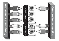
Once in the Video Setting menu, use the CURSOR ▲▼ keys to select Component (Y/Pb/Pr) if your hookup uses five (5) jacks like on the left; or select Composite (V) if your hookup uses three (3) jacks like on the right.
