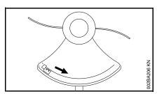
Arrows on the deflector (as seen from the underside) show the correct direction of rotation of the cutting attachment. When viewed from above, however, the cutting attachment rotates counterclockwise.
