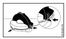
To do this with this STIHL cap, raise the grip on the top of the cap until it is upright at a 90° angle. Insert the cap in the fuel
