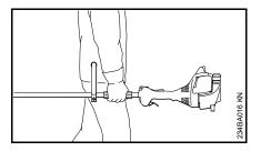
It may be carried only in a horizontal position. Grip the shaft in a manner that the machine is balanced horizontally. Keep the hot muffler away from your body and the cutting attachment behind you.
