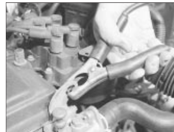
4 Connect the other end of the black jump lead to a bolt or bracket on the engine block, well away from the battery, on the vehicle to be started.
