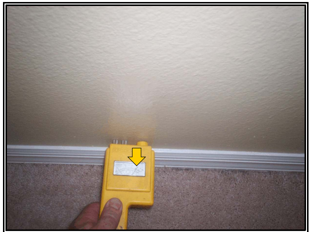
Photo 6- Increased moisture at the wall below the dining room window. The tack strip below is stained as well.
